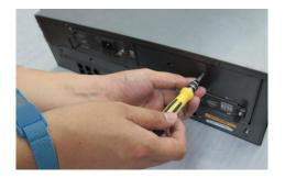
2. Insert the power module in place.
