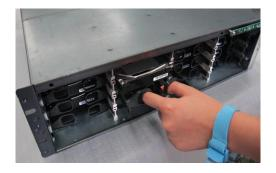
2. Remove the six fixing screws.
