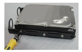
**3.** Replace the hard disk. See <u>Installing Hard Disks</u> for detailed steps.
